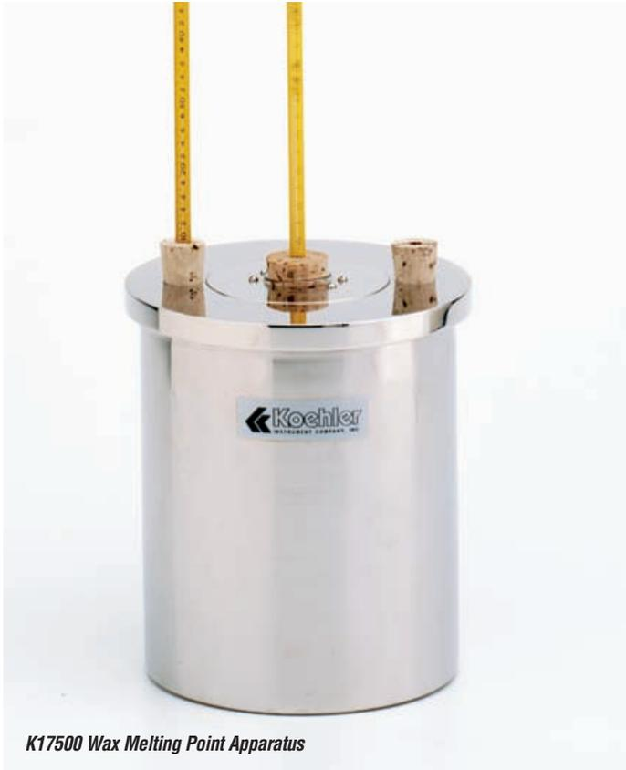
*K17500 Wax Melting Point Apparatus*
