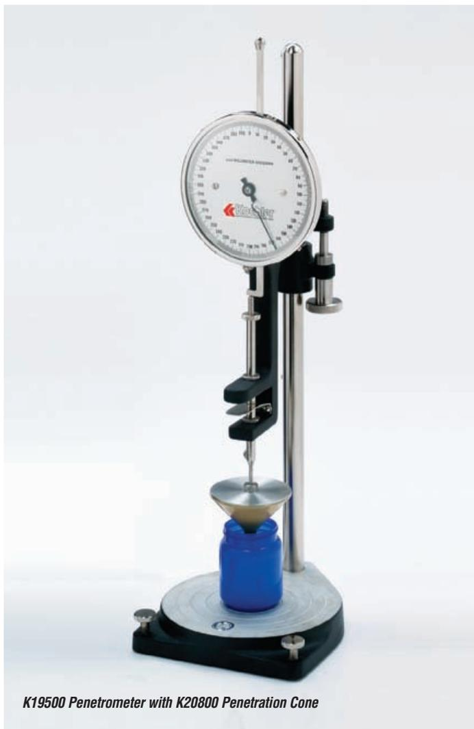
*K19500 Penetrometer with K20800 Penetration Cone*
