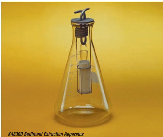
K48300 Sediment Extraction Apparatus
