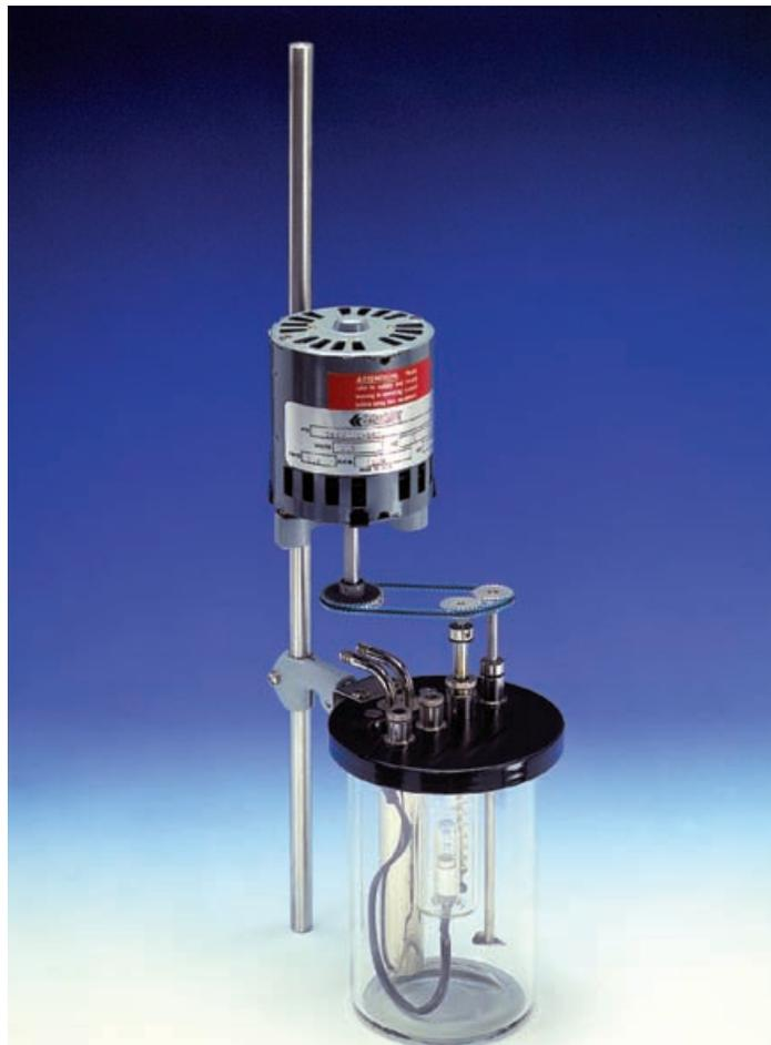
*K10190 Thin Film Aniline Point Apparatus*
