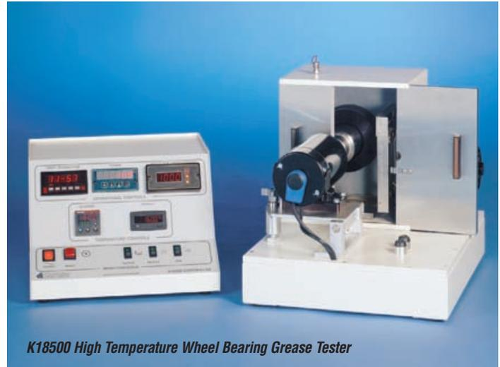
K18500 High Temperature Wheel Bearing Grease Tester
