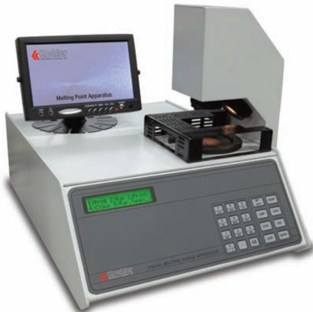
*K90190 Automatic Melting Point Range Apparatus*
