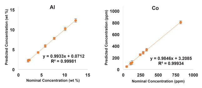
Figure 3. Multivariate calibration curves for AI (2.09 – 12.4 wt. %) and Co (49 – 820 ppm).
