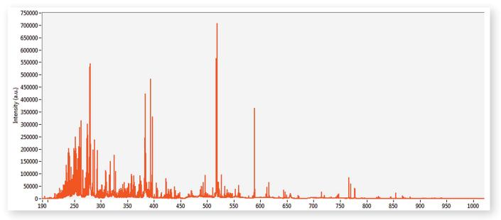
Figure 1. Typical LIBS spectrum of AMIS 171 acquired with the J200 LIBS instrument.
